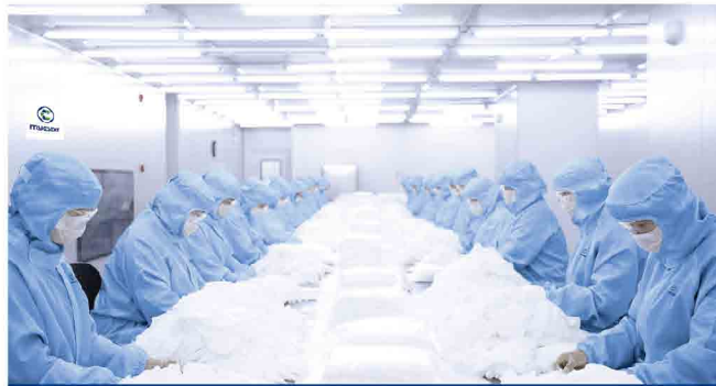
08 Full inspection of stack wiper (ENSURE APPEARANCE, QUANTITY, FLAT STACK AND VACUUM EFFECT)
