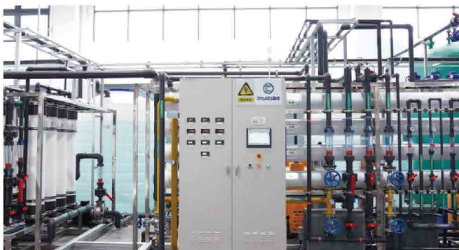
04 Ultrapure water cleaning (18.25 MΩ ULTRAPURE WATER CLEANING TO REDUCE IMPURITY AND ION CONTENT)
